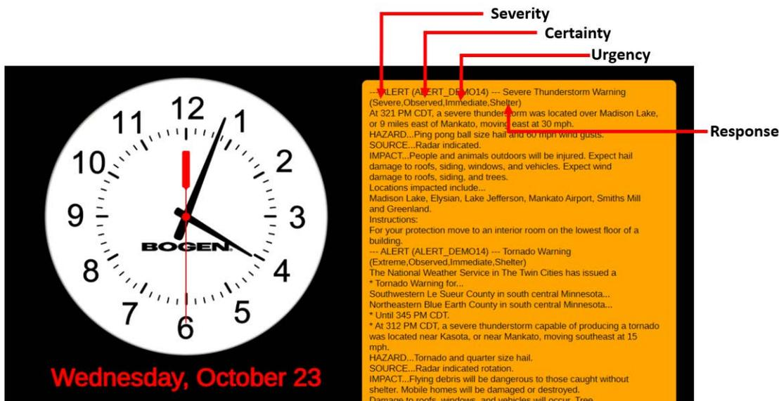
Figure 194. Sample Alert With Elements Defined
