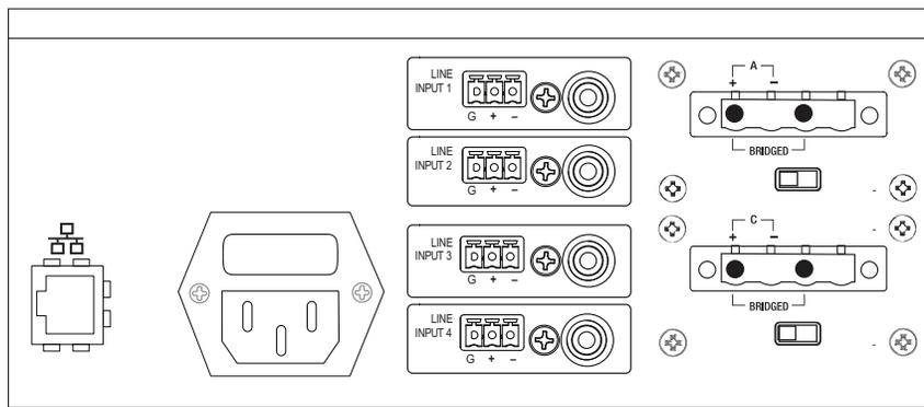
**Figure 96. Line Input for NQ-A4300-G2 Audio Power Amplifier**
