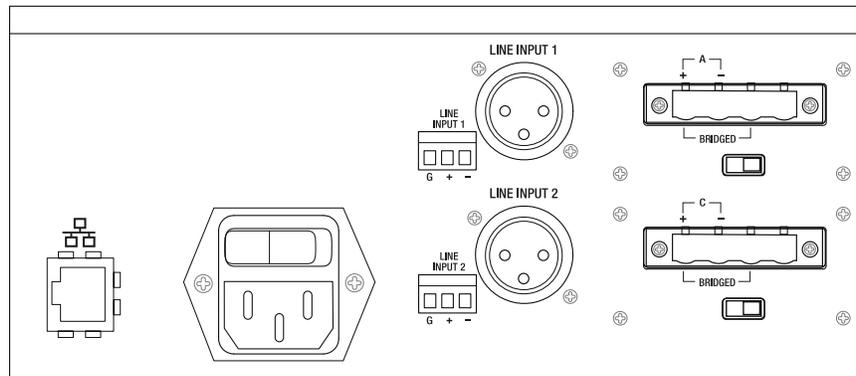
**Figure 95. Line Input for NQ-A4300-G1 Audio Power Amplifier**
