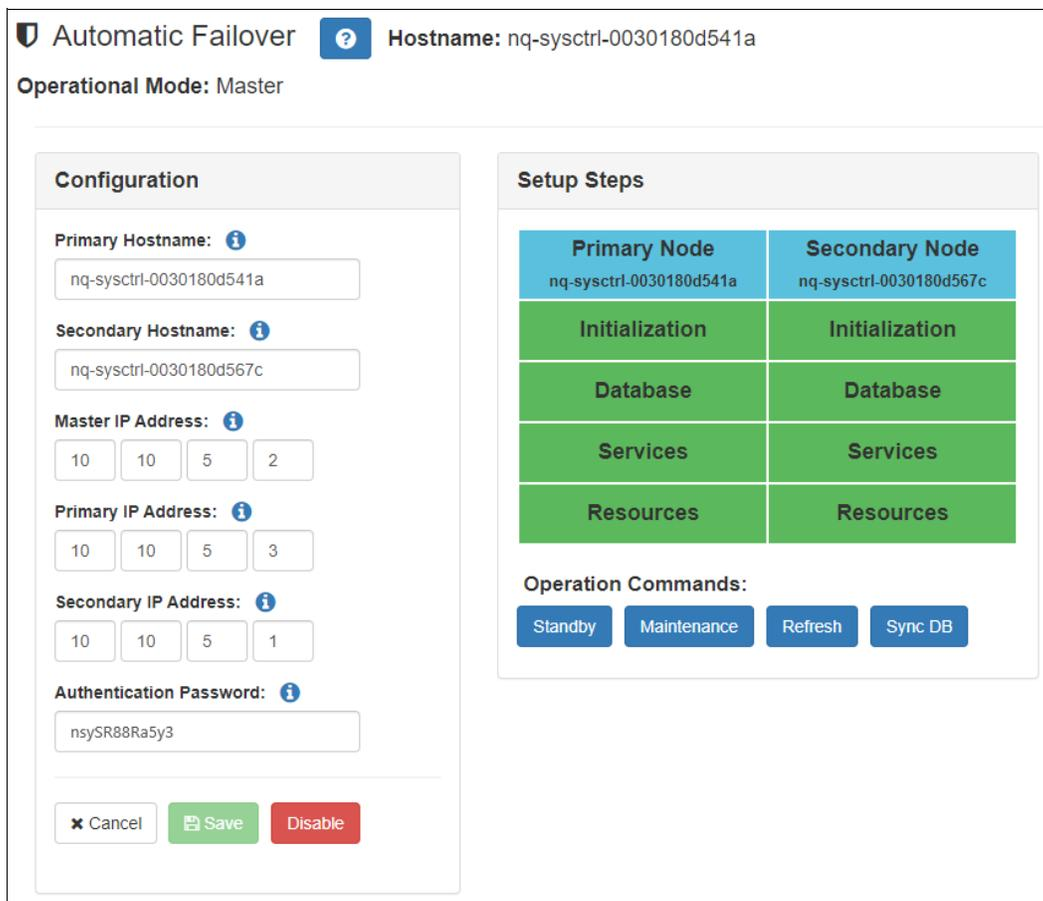
**Figure 27. Automatic Failover Operations mode**
